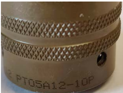
Picture 1. Colour of current MIL-SPEC connector
